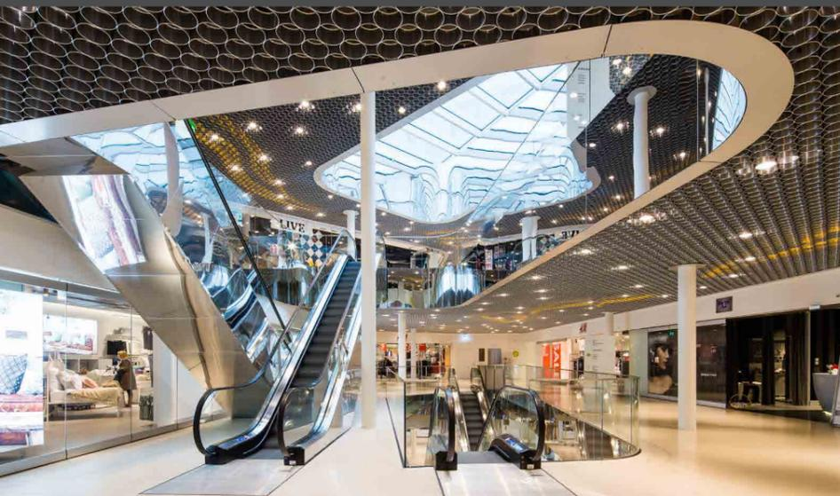
Light in the depths: numerous mirror and stainless steel surfaces reflect the light coming through the atrium roof far into the interior and offer an array of vertical vistas from the staggered galleries.
